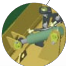
hydraulic opening rear hood
